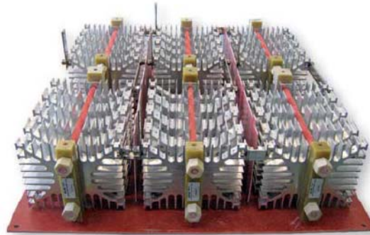
F Three Phase bridge, 4 diode for arms , full insulated clamp
