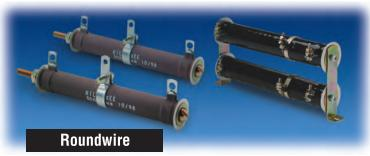
Fixed and Adjustable Roundwire resistors are available from 8 to 1150 watts. Special coatings, temperature coefficients, tolerances, and noninductive windings can be specified to meet your specific requirements.
