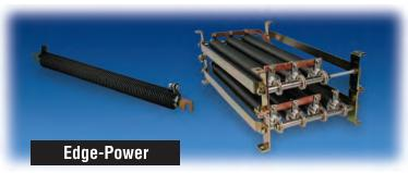
Available in sizes ranging from 400 to 1600 watts, the Edge-Power resistance ranges fit between our Ribwound and Grid Resistors. These resistors can be assembled into frames and custom enclosures which are readily available. Continuous current ratings are from 17.2 to 85 amperers.
