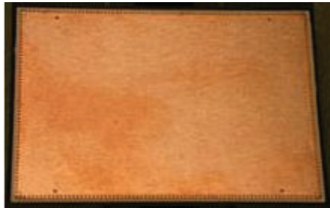
Fig. 3 - Example of discoloration
