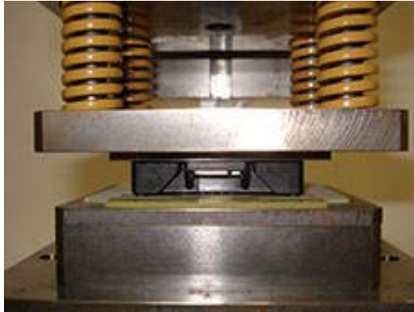
Fig. 10 - Step 3: Start the semiautomatic machine to press the pressfit module into the PCB, making sure there is no gap between the stand-off and the PCB.
