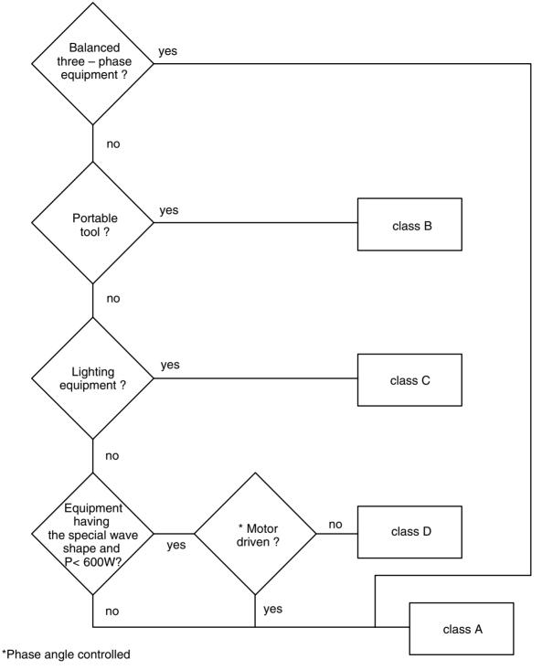
Figure 5. Flow chart for the classification of equipment
