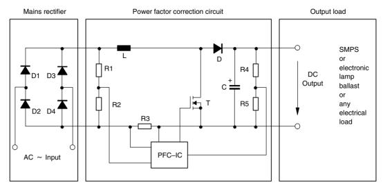
Figure 6. Typical boost converter topology for active PFC
