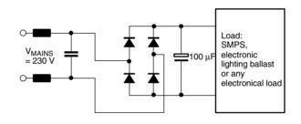
Figure 1. Standard bridge rectification of line voltage
