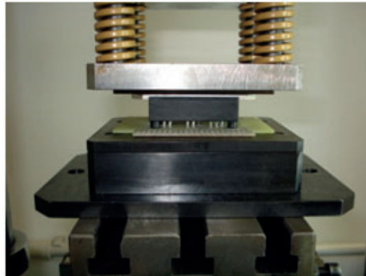
Fig. 8 - Step 3: Start the semiautomatic machine to press the press fit module into the PCB, making sure there is no gap between the standoff and the PCB
